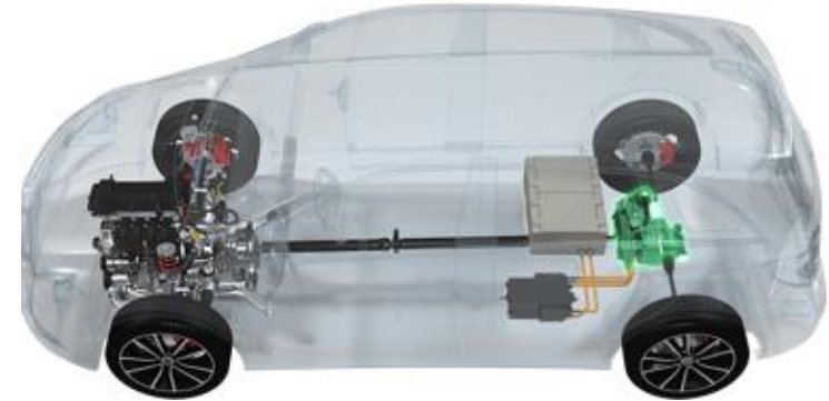
AAM P3 Rear e-Drive unit (Hybrid) Launching in 2020
